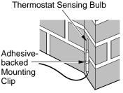
Figure 43-Locating Thermostat Sensing Bulb on Masonry Fireplace
